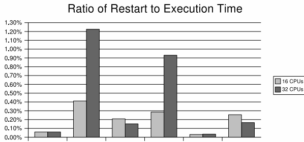
Figure 8: Restart cycles as a percentage of total execution time for TxLinux-default (SS) with 16 and 32 cpus. The percentage of restart cycles gives a theoretical upper bound on the performance benefit achievable by a scheduling policy that attempts to minimize restart waste.
